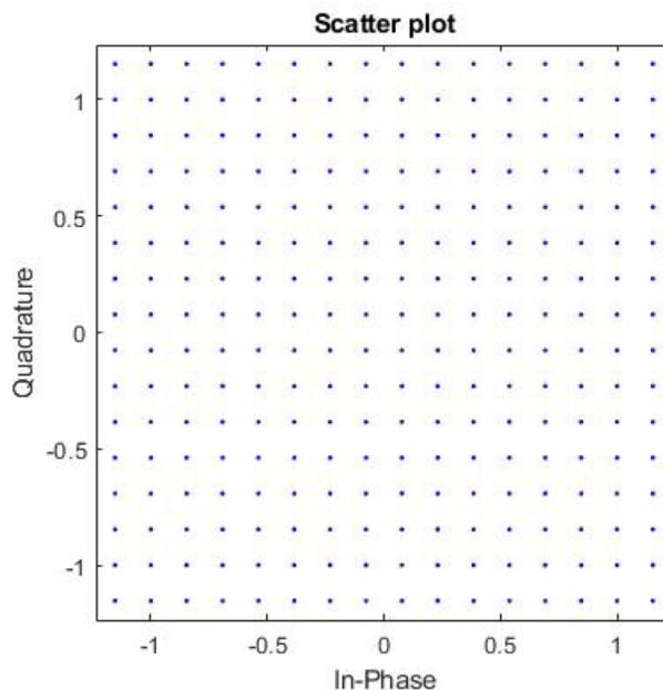
Figure 8. 256QAM constellation recovered in the receiver.
